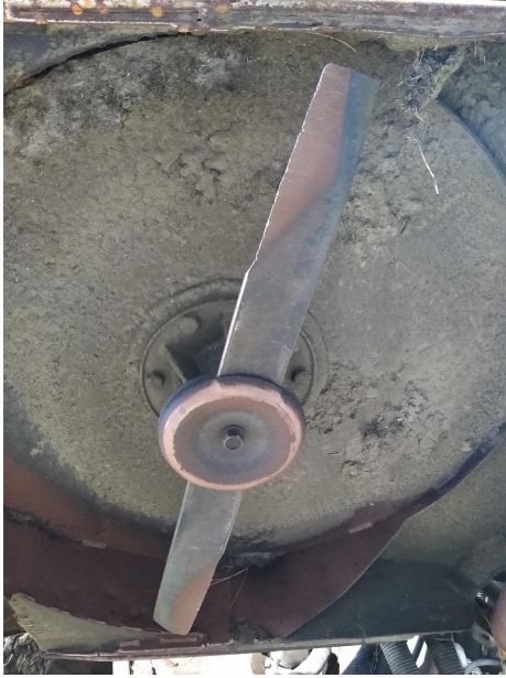
Low lift blades for thick grass in the summer
