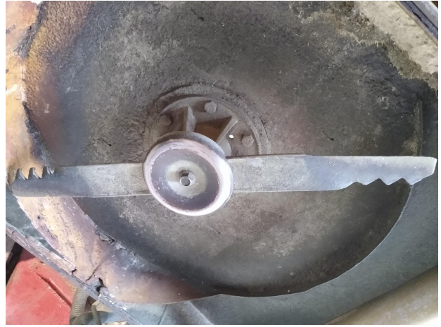
Mulching blades used during the fall.
