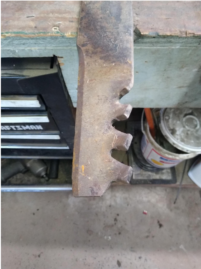
Mulching foil that chops up debris.
